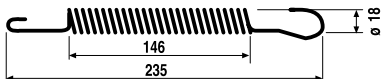
FS 010 Richiamo ceppo freno 662/100, 110/130 NC Sup. Post. 110.14 - Inf. P/A Rif. Orig. 4530055 662/100, 110/130 NC - Upper rear 110.14 lower front and rear brake block return spring Orig. Ref. 4530055 Ø 3,5
