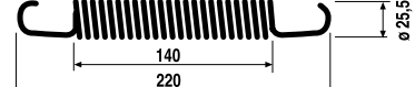
FS 009 Richiamo ceppo freno 619/300/693/697 - Ant. Post. 691/180 - Post. Rif. Orig. ★ 619/300/693/697 - front and rear; 691/180 - rear, brake block return spring Orig. Ref. ★ Ø 4,2
